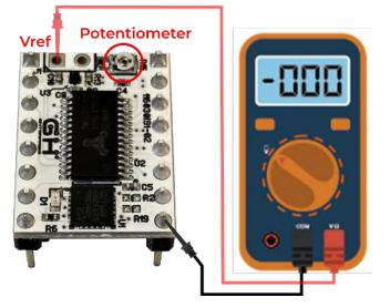
Driver motor current should match the current tolerated from your step motors. The current can be adjusted the value of VREF using the onboard potentiometer.
