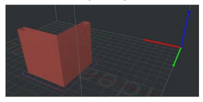
The printed part has one wall marked with X label and another one marked with Y label. The X Label is on the wall aligned along the Y axes and the Y Label is on the wall aligned along the X axis. The reason is that the ringing due to Y acceleration/deceleration are visible on X axis and vice-versa.
