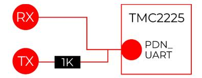
Each motion board has it custom way to enable and configure UART pins. Please refer to the user manual of your motion board. Usually instruction are referred to TMC2208. TMC2225 UART is equivalent to TMC2208.
